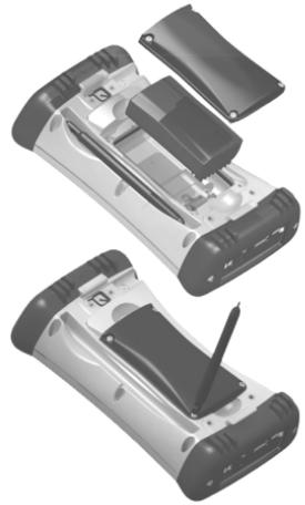
Remove the rubber cap from the end of the stylus to expose a Philips screwdriver, or use a small #1 Philips head screwdriver to finger-tighten the four screws in the battery door.
